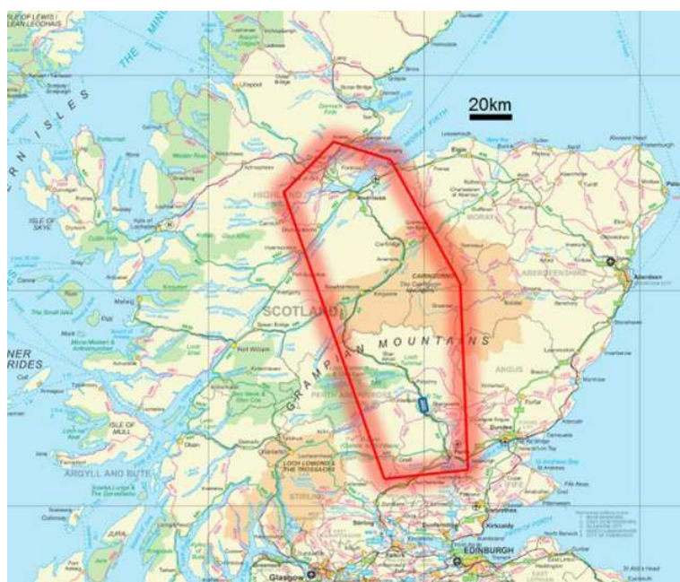
Figure 14. Three main debris flow events (blue rectangle) closed the A9 N of Dunkeld on 11 August 2004; the vulnerability shadow that was cast (bounded in red) was extensive and reflects the importance of the A9, particularly to the communities to the north. (Image based on OS 1:1,000,000 mapping. © Crown Copyright. All rights reserved Scottish Government 100020540, 2017.)
